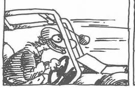
THE MASS MOVES IN A DIRECTION OPPOSITE TO THE ACCELERATION, AND THE ANGLE EVEN GIVES A MEASURE OF THE ACCELERATION.
