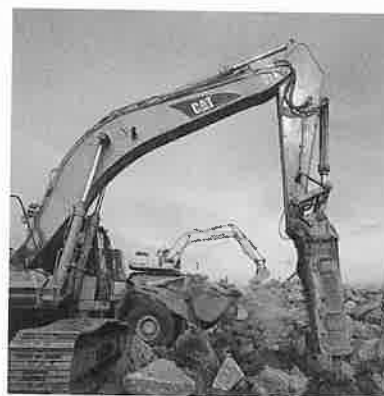
FIGURE 13.24 Pascal's principle at work in the hydraulic devices on these incredible machines. We can only wonder whether Pascal envisioned the extent to which his principle would lead to the lifting of huge loads so easily.
