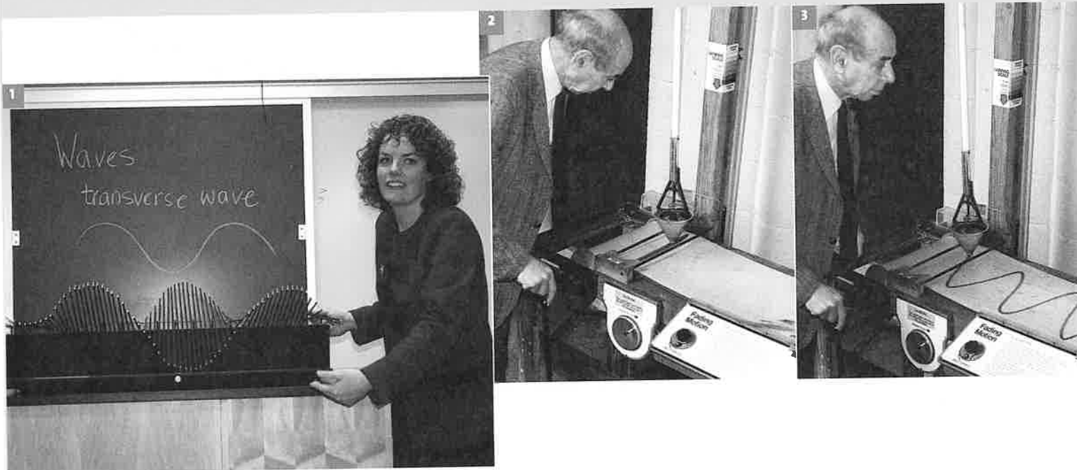
1 Diane Reindeau shows her class how waves are generated by vibrations in a classroom wave demonstrator. 2 Frank Oppenheimer at the San Francisco Exploratorium shows a straight-line trace when a swinging pendulum bob leaks sand on a stationary conveyor belt. 3 When the conveyor belt moves in uniform motion, a sine curve is traced.
