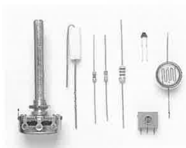
FIGURE 23.6 Resistors. The symbol of resistance in an electric circuit is \sim\sim\sim .
