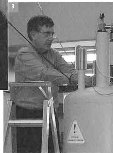
1 Fred Myers shows that the magnetic field of a ceramic magnet penetrates flesh and the plastic coating on a paper clip. 2 Ken Ganezer shows the bluish-green glow of electrons circling the magnetic field lines inside a Thomson tube. 3 Paul Callaghan is about to load a nuclear magnetic resonance sample into the room temperature bore of a 7 Tesla superconducting magnet at Victoria University of Wellington in New Zealand.
