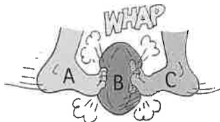
FIGURE 5.13 Both A and C act on B. They can cancel each other, so B does not accelerate.
