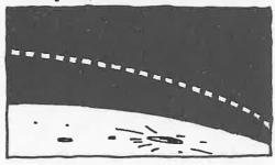
EVENTUALLY, AS I FIRE FASTER AND FASTER, BY THE TIME THE BULLET HAS FALLEN 4 FT., THE GROUND HAS CURVED 4 FT. DOWN AND THE BULLET 15 **STILL**4 FT. HIGH! BY THE TIME IT
